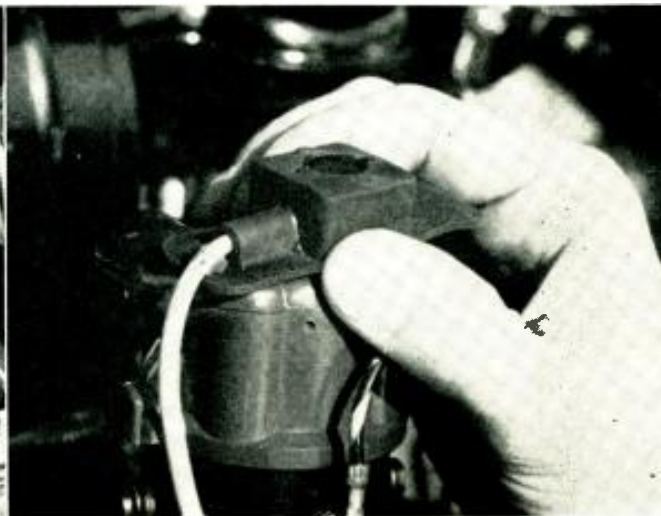
The contact mike offers the sports car enthusiast a means of checking the performance and timing of his mill. Left, the mike is held on the generator and right, is shown on the distributor cap. Mike must be held firmly in place or taped down to avoid introduction of extraneous noises.
